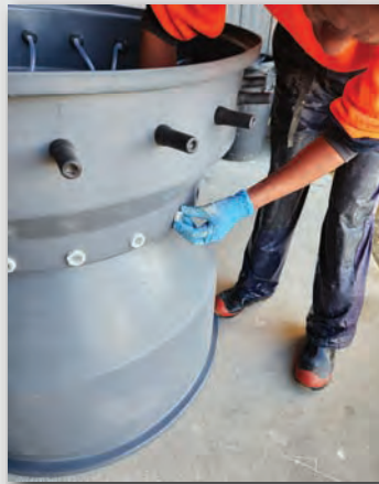
As the teats start to wear, transition the teats to the top of the feeder. Put the blanking plugs to seal the bottom holes.
